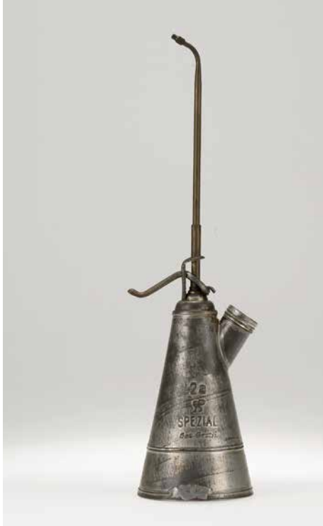
The first pump oiler invented by Jakob Preßl in 1914
